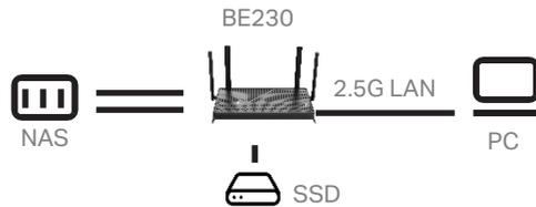
The test PC should install an SSD (solid-state drive), or a **2.5G or above** Ethernet adapter.
