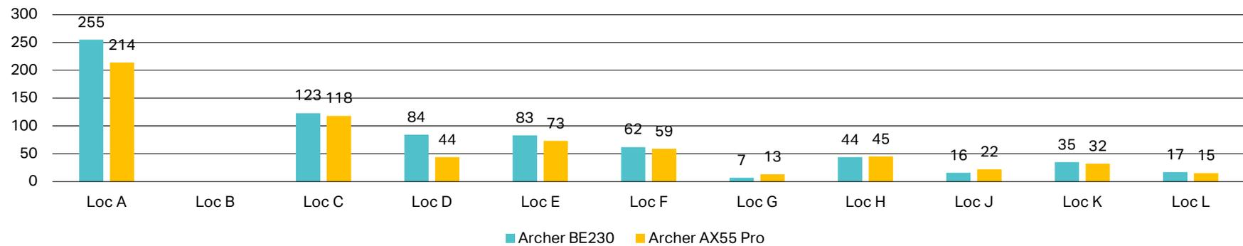
\*Archer BE230 features two lateral 2.4G antennas, distinct from Archer AX55 Pro. This design may lead to differences in 2.4G Wi-Fi upload performance at various locations compared to Archer AX55 Pro.
