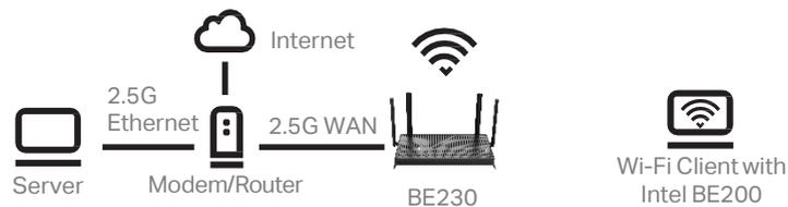
If the Modem/Router doesn't support 2.5Gbps Ethernet, please connect the Server to the router's 2.5Gbps LAN port instead.
